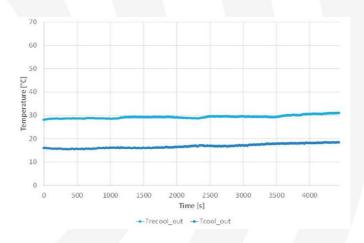
*Fig.* 10. *Fluid temperatures measured at the adsorption machine external circuits: re-cooling (cyan) and cooling (blue).*
