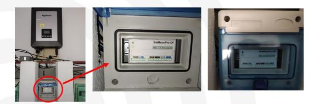
Fig. 24. BatMeter device.
