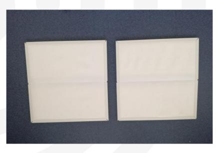
*Fig.* 14. *Radiative Cooling panels for extracting potable water from dew.*
