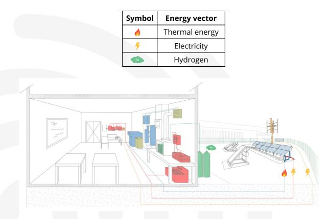
*Fig. 1. Representation of the hybrid energy system implemented at CISE | GIRS-RES.*
