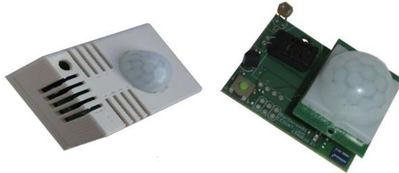
BatSense device including temperature, humidity, luminosity and presence sensors
