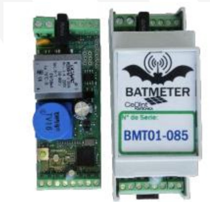
BatMeter device (PCB board and DIN encapsulation)
