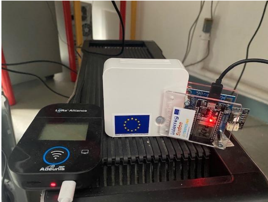
Joint deployment of neOSensor devices and Elsys ERS devices in an L3i office room
